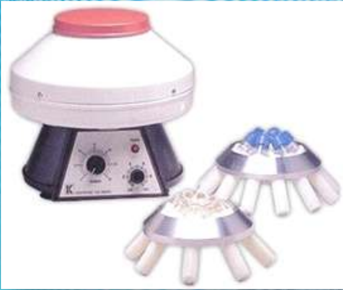
BENCH TOP CENTRIFUGE MODEL - PLC-03 CAPACITY - 8 X 15ML ROTOR - A-01815 MAX RPM - 1000 - 4000 RCFXG - 2422 SUGGESTED TUBES FX12MM CONICAL
